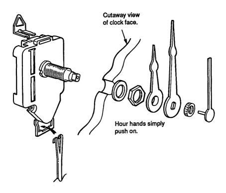
To achieve the proper pendulumlength simply cut, or snap, along the appropriate groove.
