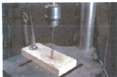
Figure 5: An easy way to center a dowel below a small drill bit is to first clamp scrapwood to your drill press table and drill a hole to fit the dowel.
