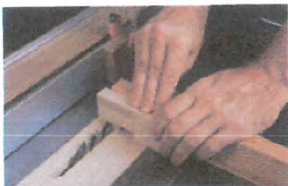
Figure 4: Use a 1/2" dado blade to cut notches for the rear wheels in the truck base. Make several passes, and use a set-up block to limit the cuts.
