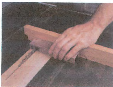
Figure 3: Lay out the posts and overall length of the cab, then support the stock with your miter gauge while clearing the remaining waste.
